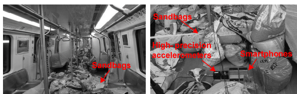
Fig. 4 Field test setup
