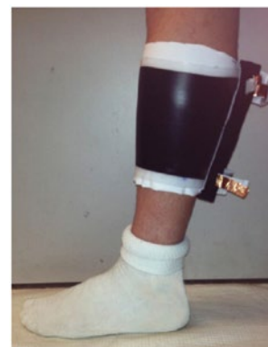
Fig. 4 A DE actuator for lower extremity (human calf) rehabilitation (Reprinted from Pourazadi et al. (2014), Copyright 2014, with permission from IOP Publishing Ltd.)
