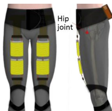
Fig. 10 A stretching-type structure PVC gel actuator for walking assistance (Reprinted from Li and Hashimoto (2016), Copyright 2016, with permission from Elsevier)
