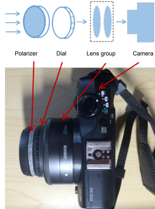
Fig. 2 Photograph and configuration of the polarized camera device
