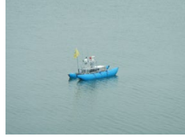
Fig. 3 An unmanned surface bathymetry vehicle (USBV)
