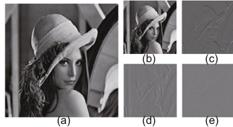
Fig. 4 One-level DWT decomposition: (a) original image of size M \times N ; (b) approximation band of size (M/2) \times (N/2) ; (c) horizontal band of size (M/2) \times (N/2) ; (d) vertical band of size (M/2) \times (N/2) ; (e) diagonal band of size (M/2) \times (N/2)
