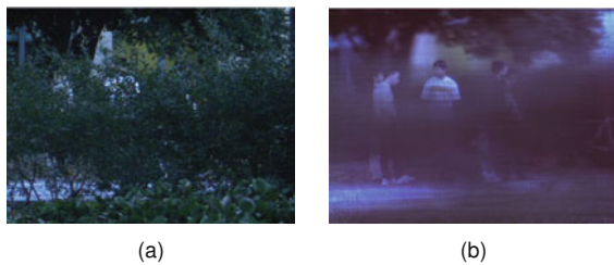
Fig. 8 Seeing through occlusion (Vaish, 2007): (a) image from one view; (b) synthetic aperture image
