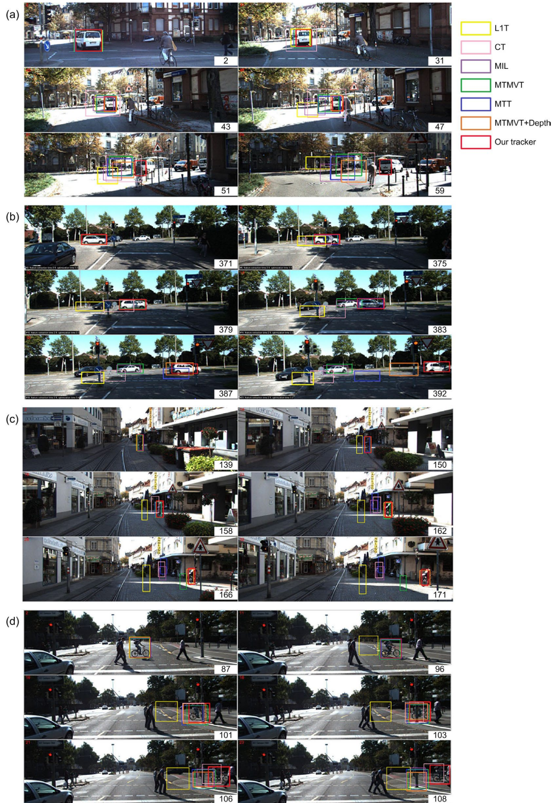
Fig. 5 Comparisons of the tracking results on the KITTI Vision benchmark: (a) training_00 (frames 2, 31, 43, 47, 51, 59); (b) training_01 (frames 371, 375, 379, 383, 387, 392); (c) training_13 (frames 139, 150, 158, 162, 166, 171); (d) training_15 (frames 87, 96, 101, 103, 106, 108) (References to color refer to the online version of this figure)
