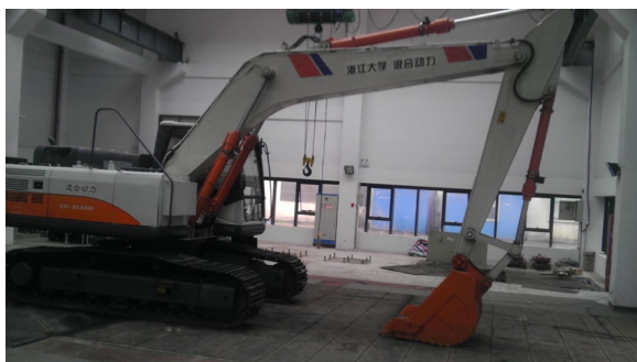
Fig. 9 Hybrid excavator with the electric swing system
