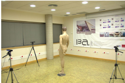
Fig. 3 Photograph of the experiment performed with three sensors. Sensors 1 and 2 were positioned perpendicular to each other, sensors 2 and 3 were also perpendicular to each other, and sensors 1 and 3 were facing each other
