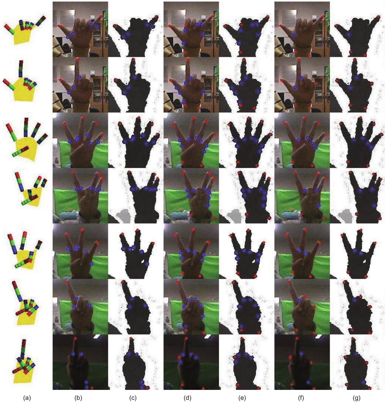
Fig. 10 Qualitative results of hand articulations of Experiment 1 (red: fingertips; blue: finger-valleys): (a) hand models generated by our method; (b) and (c) the CSS phase; (d) and (e) the K-cos method (Lee and Lee, 2011); (f) and (g) the convex-hull method (Nagarajan et al. , 2012). Three or four fingers are bending, or the thumb is bending. References to color refer to the online version of this figure
