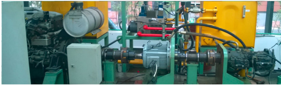
Fig. 17 Experimental platform of the HHE power transmission system
