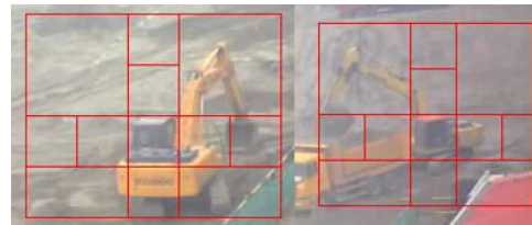
Fig. 5 Expanding a patch's contour (the cab is the goal part and the array R is [2.0, 2.0, 2.0, 1.0] )
