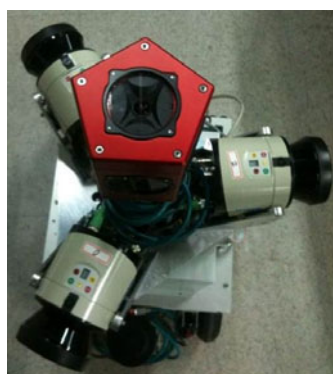
Fig. 5 Three SICK LMS-151 laser scanners and a PointGrey Ladybug 3 panoramic camera integrated in an RGB-D unit
