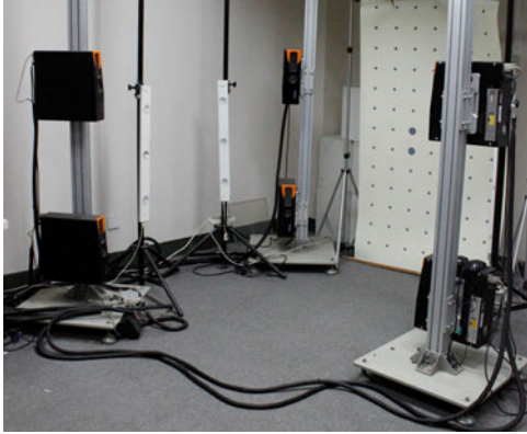
Fig. 2 The scanner 3D Mega Capturor II LF (InSpeck Inc., Canada)
