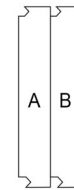
Fig. 26 Stacking of part B from the right side of part A (the bottom-left corner of part B's bounding box coincides with the bottom-right corner of part A's bounding box)
