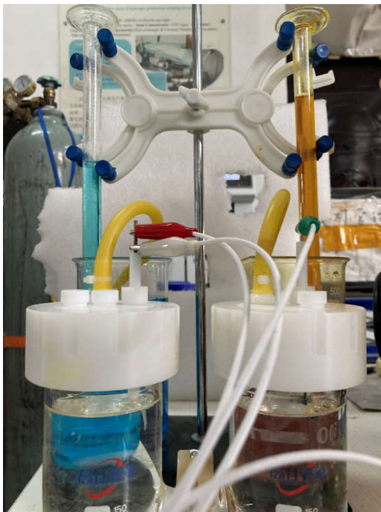
Fig. S10 Physical image of Faradic efficiency (FE) testing device.
