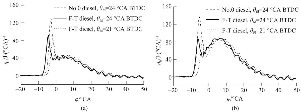
**Fig. 2** Comparison of heat release rate between F-T and No. 0 diesel fuels at  $n = 1800$  r/min
