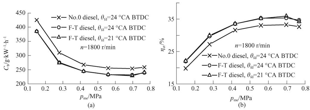
**Fig. 5** Brake specific fuel consumption and effective thermal efficiency of F-T and No. 0 diesel fuels
