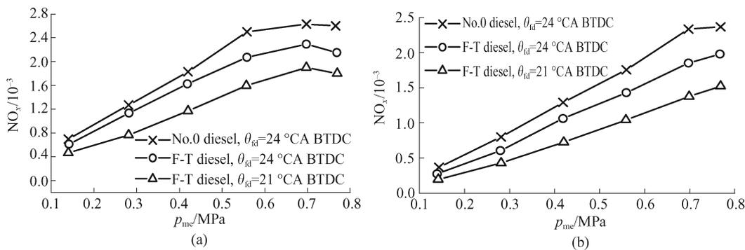
Fig. 8 Comparison of  $\text{NO}_x$  emissions between F-T fuel and No. 0 diesel fuel (a)  $n = 1200$  r/min; (b)  $n = 1800$  r/min
