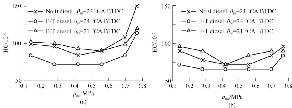
Fig. 6 Comparison of HC emissions between F-T fuel and No. 0 diesel fuel (a)  $n = 1200$  r/min; (b)  $n = 1800$  r/min
