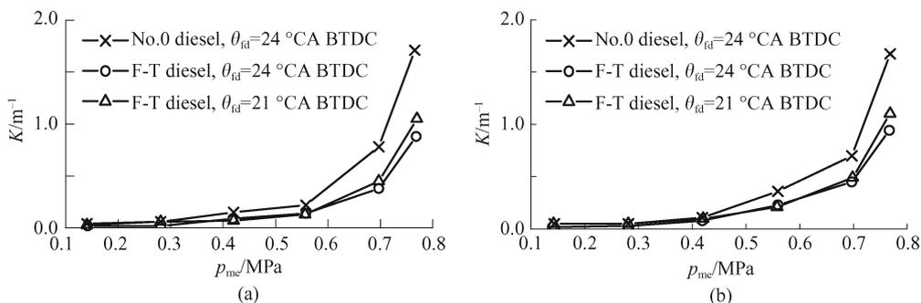
Fig. 9 Comparison of smoke emissions between F-T fuel and No. 0 diesel fuel (a)  $n = 1200$  r/min; (b)  $n = 1800$  r/min
