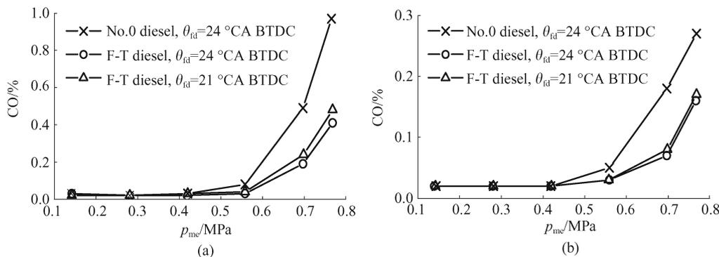
Fig. 7 Comparison of CO emission between F-T fuel and No. 0 diesel fuel (a)  $n = 1200$  r/min; (b)  $n = 1800$  r/min
