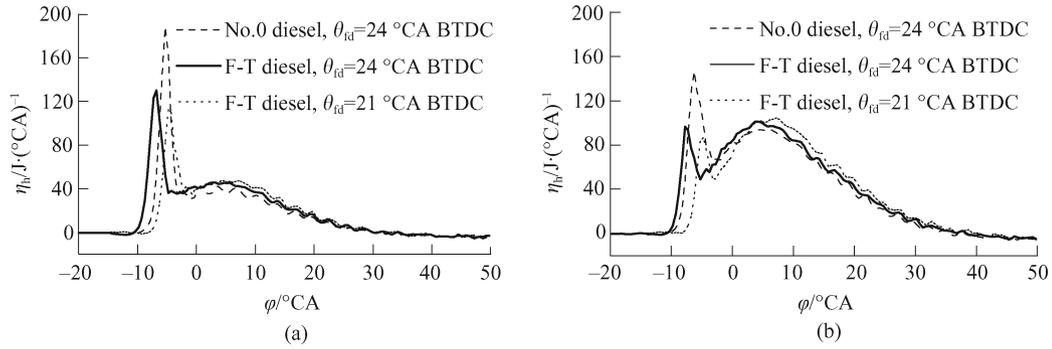
**Fig. 1** Comparison of heat release rate between F-T and No. 0 diesel fuels at  $n = 1200$  r/min
