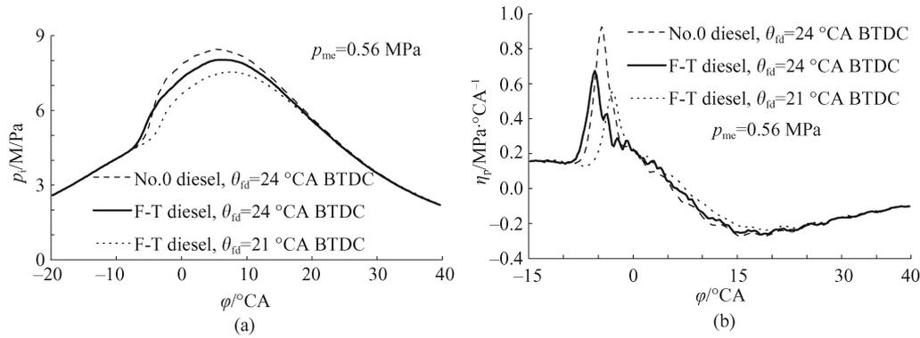
**Fig. 4** Comparison of in-cylinder pressure and rate of pressure rise between F-T fuel and No. 0 diesel fuel at  $n = 1800$  r/min
