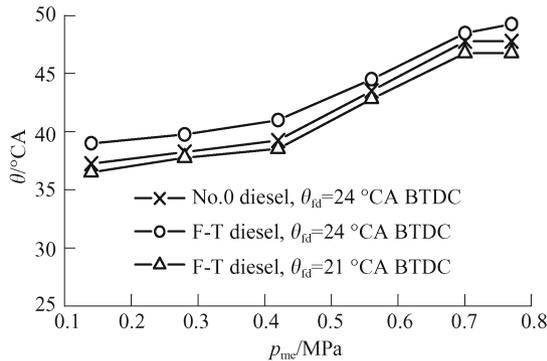
**Fig. 3** Comparison of combustion duration between F-T fuel and No. 0 diesel fuel at  $n = 1800$  r/min
