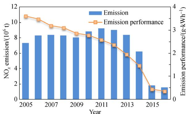
**Fig. 5** Emission and its performance of NO<sub>x</sub> of coal-fired power plants in China
