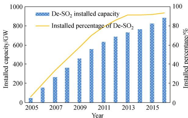
Fig. 2 Installed capacity and its percentage of De- $\text{SO}_2$  of coal-fired power plants in China
