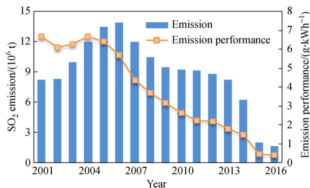
Fig. 3 Emission and its performance of  $\text{SO}_2$  of coal-fired power plants in China
