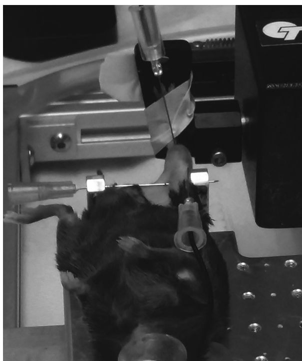
Figure 2 Force transducer measurement. The mouse is anesthetized and its foot attached to the pedal of the force transducer. An electrode is placed over the tibialis anterior muscle. A second electrode is placed at the base of the tendon. An electrical current stimulates the muscle to contract. As the muscle contracts, the mouse pushes the pedal, and the resulting force is recorded.
