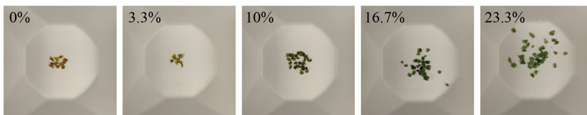
Figure S2. Pictures of dried chitosan-MMT nanocomposites of different MMT contents.
