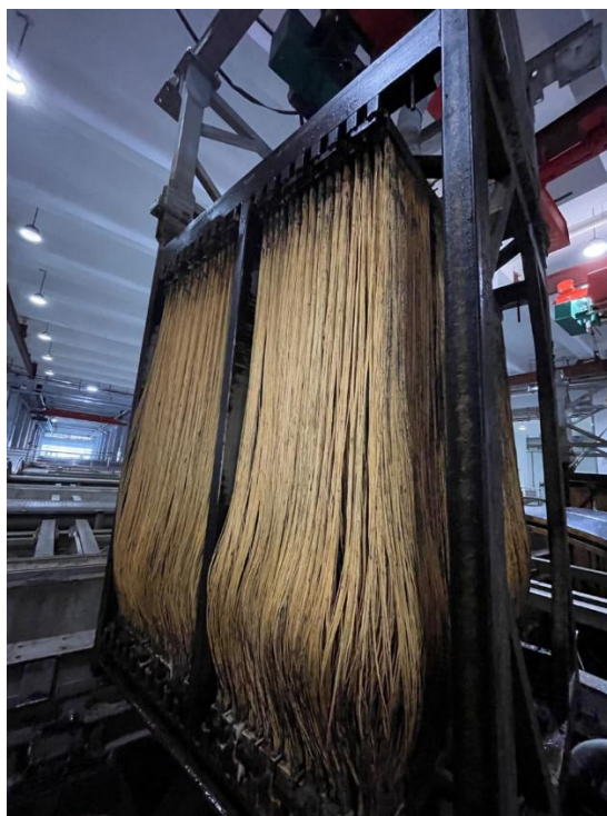
Fig. S3. The on-site photo of the fouled membrane module showing the spatial heterogeneity of foulant deposition.
