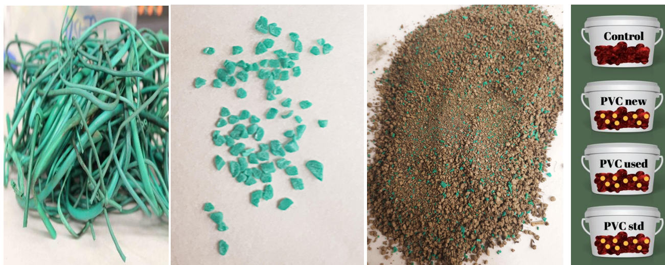
Figure S1 Plastic PVC ties (A) collected from the sampled vineyard have been grinded into random size of micro-PVC particles Figure (B) shows the micro-PVC fragments of irregular size that were sieved through a 1-mm sieve. The micro-PVC particles were inoculated into the soil sample (C) and homogeneously mixed at a concentration of 1% (w:w). In design of experiment we used control soil sample (no plastic addition), PVC new (microplastic from new PVC tie), PVC used (microplastic from collected PVC ties from vineyard) and PVC std (PVC microplastic purchased from Sigma Aldric). 120 days of incubation was done on calcareous and acid soil samples.
