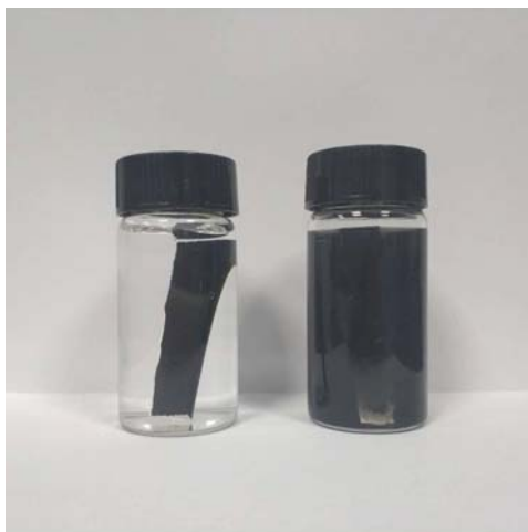
Fig. S2 The digital picture of cross-linked and non-cross-linked CNTs/ceramic membrane after 30 min ultrasonic shock
