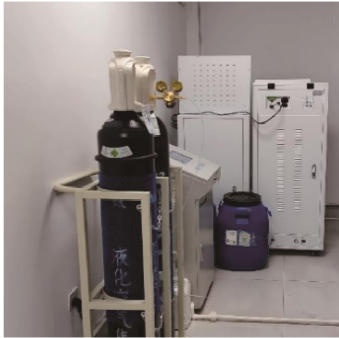
Fig. S3. The picture of surface water quality monitoring with the automatic water toxicity determination system in Shangqiankou station.
