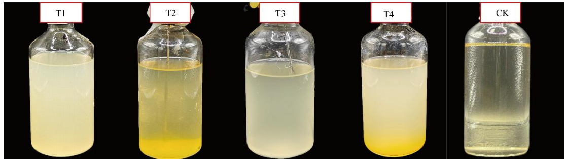
Figure S2 Experimental phenomena of cultures under different As contaminants during incubation. T1, T2, T3 and T4 reactors contain 5 \text{ mg L}^{-1} As (V), 75 \text{ mg L}^{-1} As (V), 0.7 \text{ mg L}^{-1} As(III) and 10 \text{ mg L}^{-1} As(III), respectively, and CK represents the control groups with sterilized culture.
