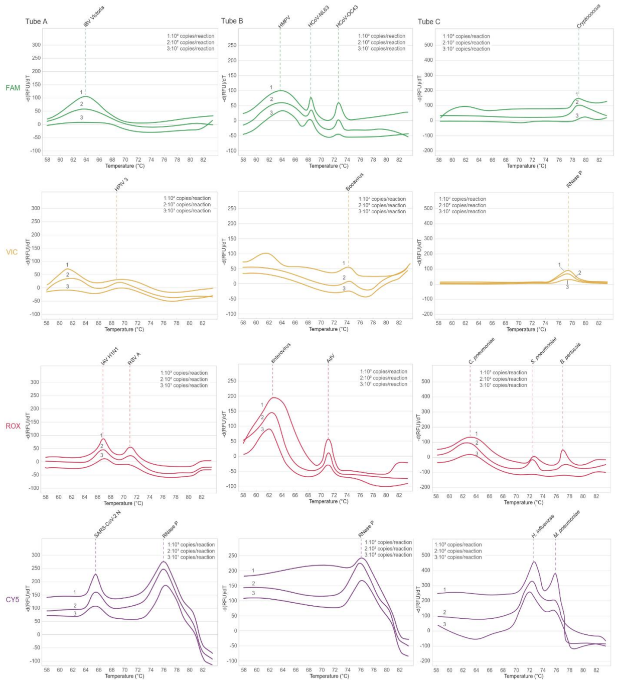
Fig. S3 Concurrent real-time PCR and melting curve analysis in three tubes. Nucleic acid reference material of 17 species (IBV Victoria, HMPV, HCoV-NL63, HCoV-OC43, Cryptococcus , HPV-3, Bocavirus, IAV H1N1, RSV A, Enterovirus, AdV, C. pneumoniae , S.pneumoniae , B. pertussis , SARS-CoV-2 N, M. pneumoniae , H. influenzae ) were quantitated by determination of the quantification cycle (C q value) that occurred during real-time PCR, and were each identified by the unique combination of the fluorescent color and the T m value of their melting peak at 5 × 10 3 , 5 × 10 2 , 5 × 10 1 , 5 × 10 0 copies/reaction.
