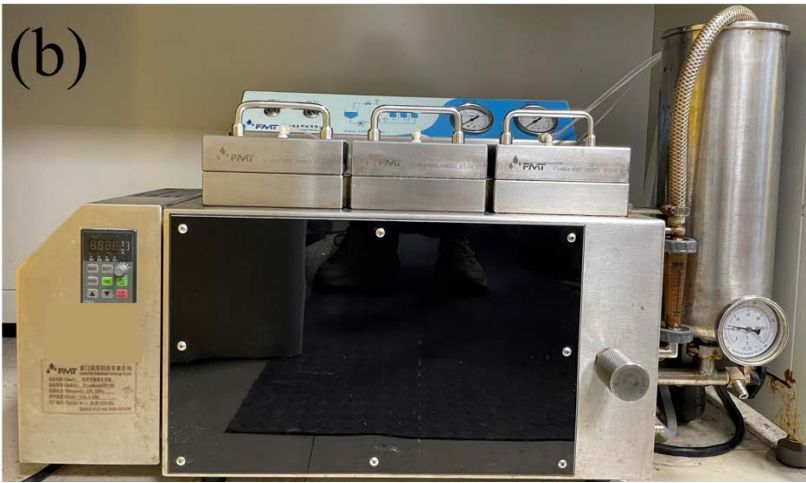
Fig. S1 (a) The automatic film applicator. (b) The triple high pressure flat membrane test equipment.
