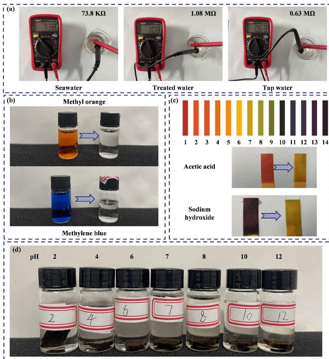
Fig. S3. (a) Electrical resistance of seawater, purified water and tap water. (b) Digital photographs of methyl orange (MO) and methylene blue (MB) solutions before and after purification. (c) pH values of acetic acid and NaOH solutions before and after purification. (d) Digital photographs of PVV@VLJ-LIS after immersion in solutions with different pH values for 72 h.
