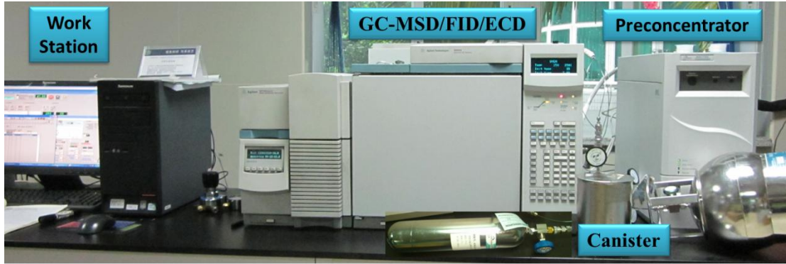
Fig. S7. The preconcentrator coupled with a Gas Chromatograph/Mass Selective Detector/Flame Ionization Detector/Electron Capture Detector (GC-MSD/FID/ECD)
