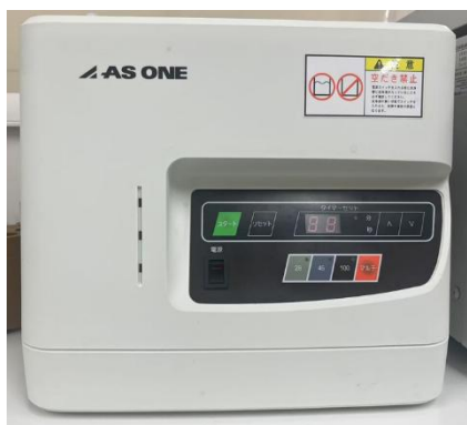
Fig. S1 Experiment setup photograph for catalytic degradation. Ultrasound bath working conditions: 45 kHz, 100 W.
