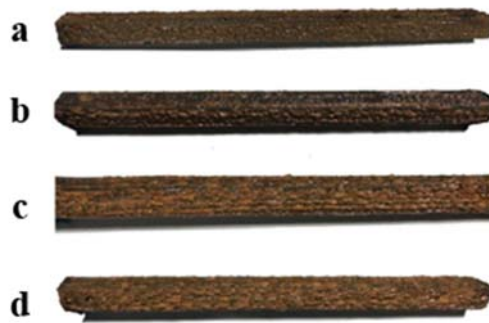
Fig. S8 Photographs of coupons in BAR during the test period. (a), (b), (c) and (d) were taken in week 2, 4, 6, and 8.
