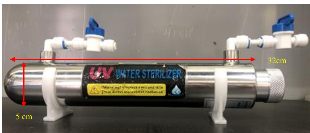
Figure S1. Diagram (top) and real picture (bottom) of the UV/VUV photoreactor used in this study. The reactor was placed horizontally. Outlet (1) was used for samples retrieving. Inlet (3) was used for purging N 2 .
