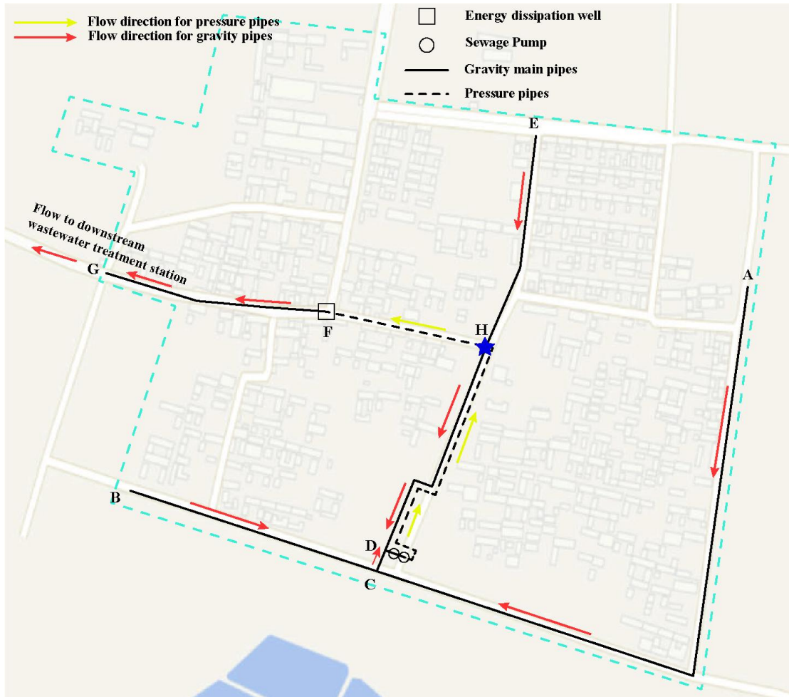
Figure. S1 Sewer pipe distribution
