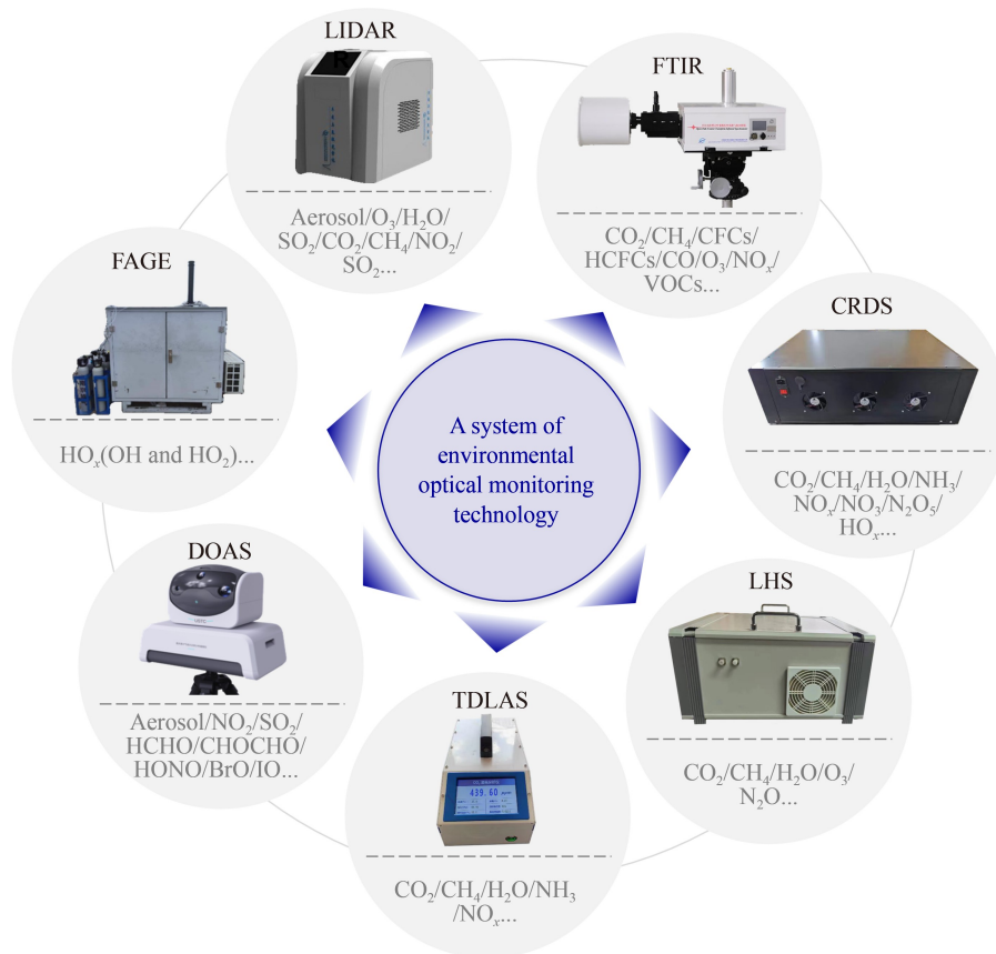
Fig. 1 Environmental optical monitoring system.
