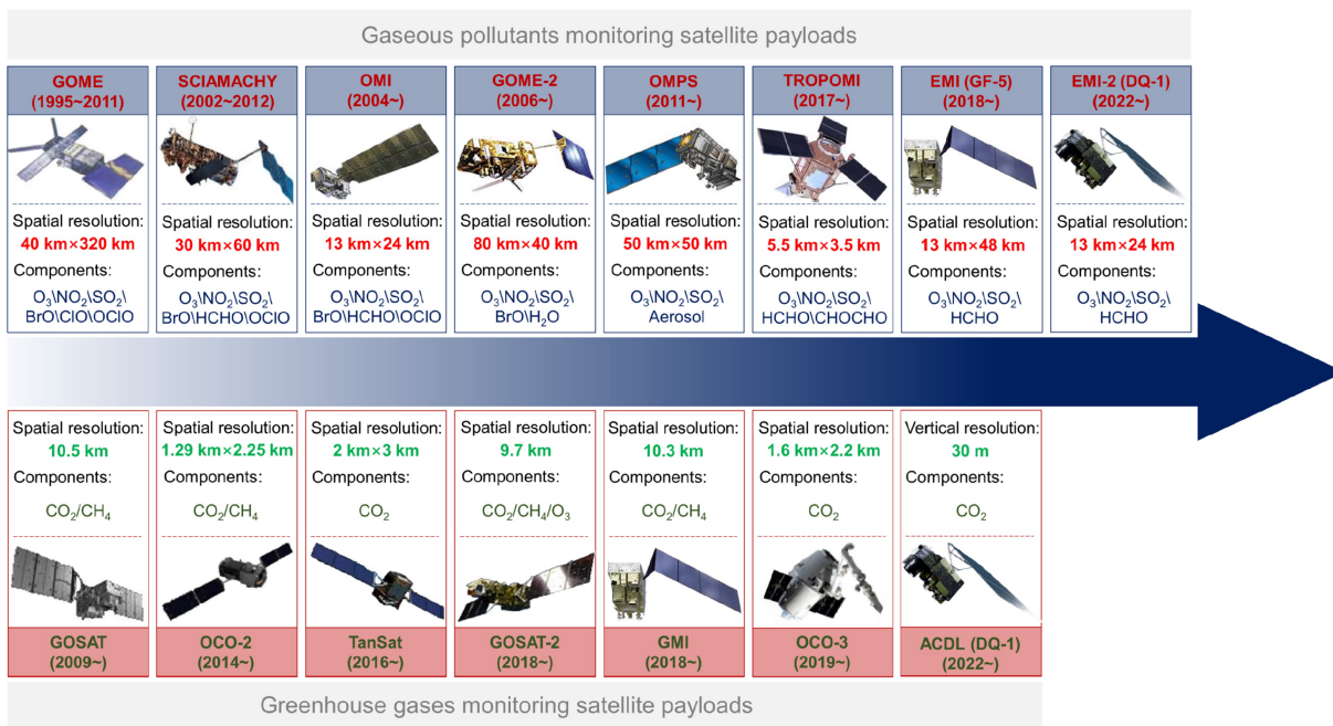
Fig. 2 History of the development of hyperspectral remote sensing satellites for pollutants and greenhouse gases.
