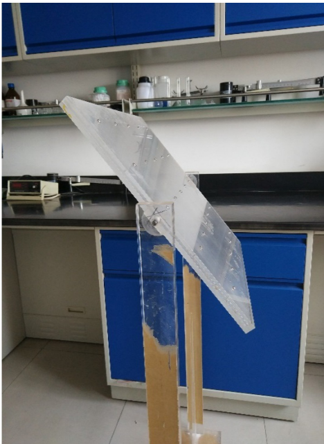
Fig. 3 Physical simulation of carbon dioxide flooding.
