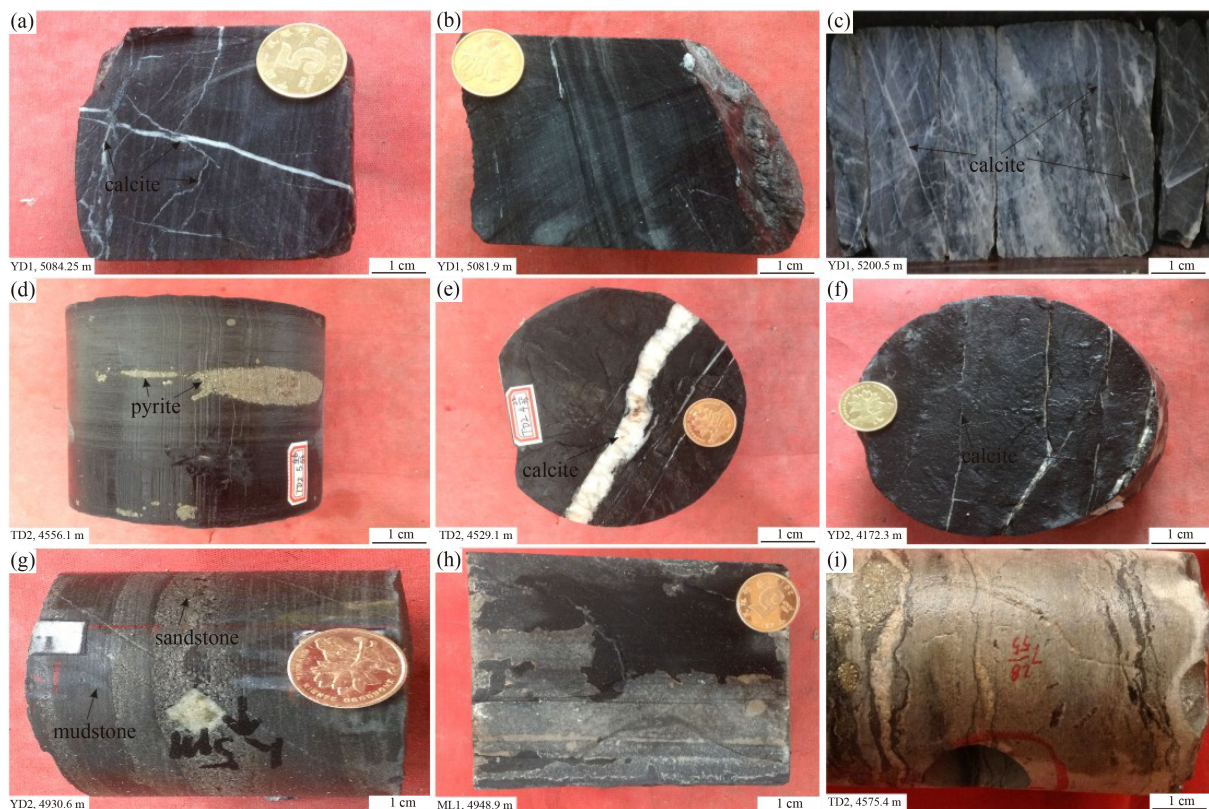
Fig. 9 The summary of cores showing the characteristics of platform facies during depositional period of the Cambrian-Ordovician in eastern Tarim Basin. (a) Middle Cambrian, limy mudstone filled with calcite; (b) Middle Cambrian, carbonaceous mudstone; (c) Middle Cambrian, gray micrite; (d) Yijianfang Formation and Yingshan Formation, grayish black mudstone filled with pyrite; (e) Yijianfang Formation and Yingshan Formation, black mudstone filled with calcite; (f) Tumuxiuke Formation, black carbonaceous mudstone filled with calcite; (g) Lower Cambrian, dark gray and black mudstone, gray medium-to fine-grained sandstone; (h) Tumuxiuke Formation, black limy mudstone filled with calcite; (i) Penglaiba Formation, gray micrite filled with pyrite and boulder clay.
