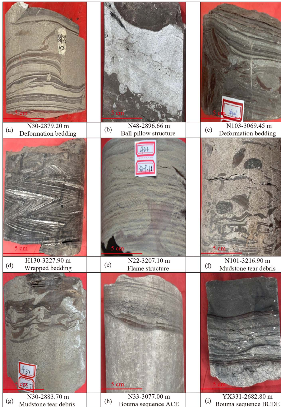
Fig. 6 Sedimentary structure. (a) N30-2879.20 m, Deformation bedding; (b) N48-2896.66 m, Ball pillow structure; (c) N103-3069.45 m, Deformation bedding; (d) H130-3227.90 m, Wrapped bedding; (e) N22-3207.10 m, Flame structure; (f) N101-3216.90 m, Mudstone tear debris; (g) N30-2883.70 m, Mudstone tear debris; (h) N33-3077.00 m, Bouma sequence ACE; (i) YX331-2680.80 m, Bouma sequence BCDE.
