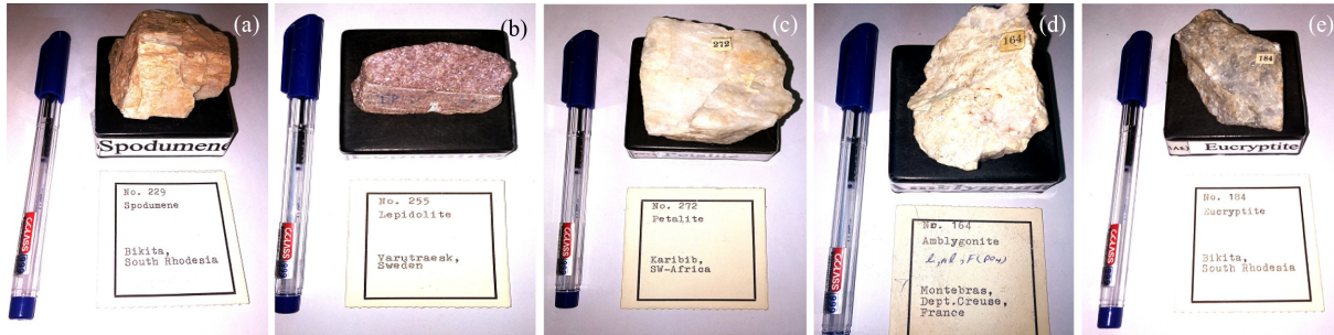
Fig. 2 The studied LCMs available in the mineralogical museum of the Department of Geology: (a) spodumene, (b) lepidolite, (c) petalite, (d) amblygonite, and (e) eucryptite.
