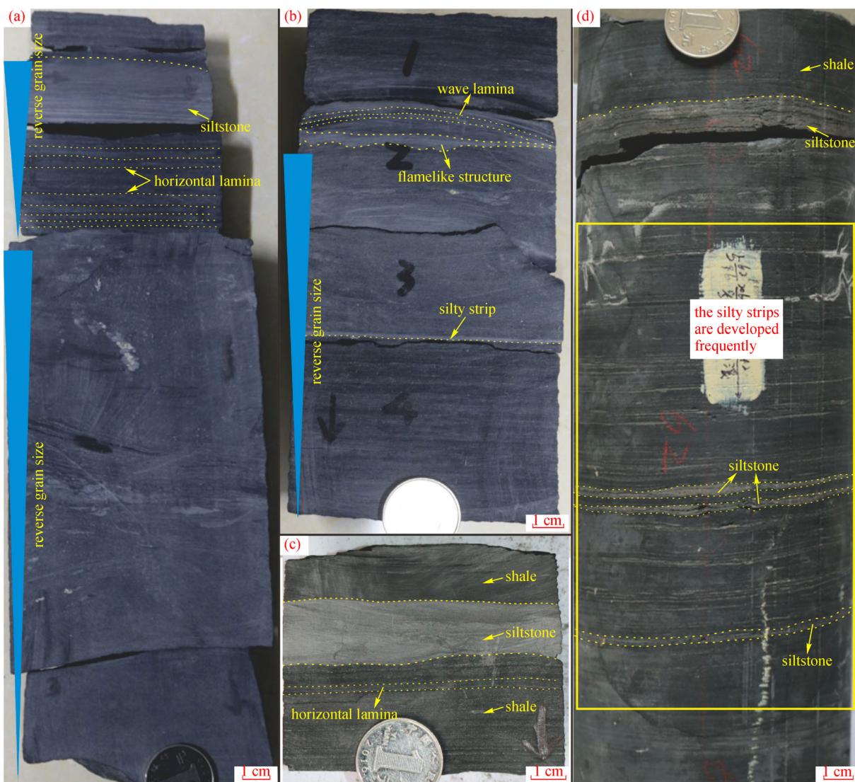
Fig. 3 Macroscopic characteristics of the siltstone-mudstone rhythmic sedimentary sections in the Lower Member of the Longmaxi Formation from the N2 well and N3 well. (a): Horizontal laminae developed in shale layer, 3124.63–3124.93 m, N2 well; (b): Wave laminae developed in siltstone layer, 3105.04–3105.30 m, N2 well; (c): Shale and siltstone are in direct sharp contact, 3131.17–3131.52 m, N2 well; (d): Silty strips had developed in high frequency, 2063.15–2063.42 m, N3 well.
