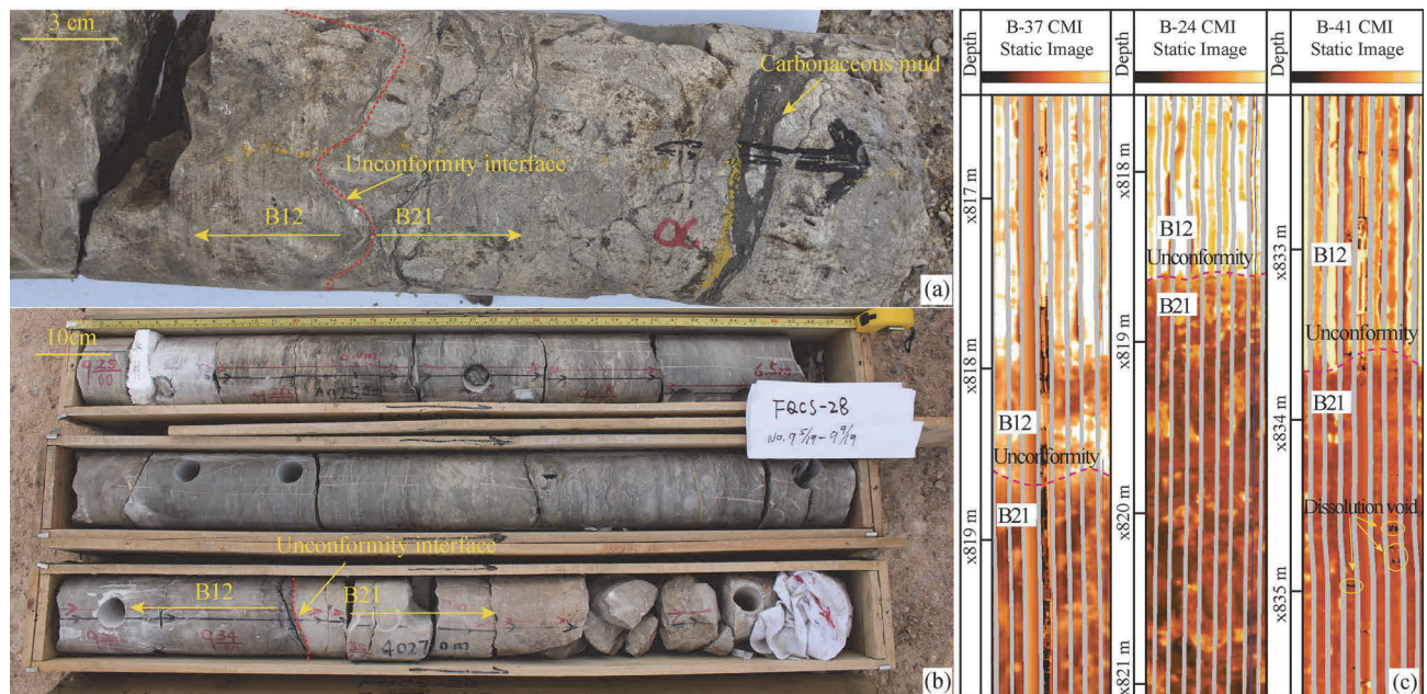
Fig. 2 Core karst unconformity features of the Mishrif Formation in the Missan Oil Fields. (a) Well B-22; (b) Well F-28; (c) Wells B-37, B-24 and B-41.
