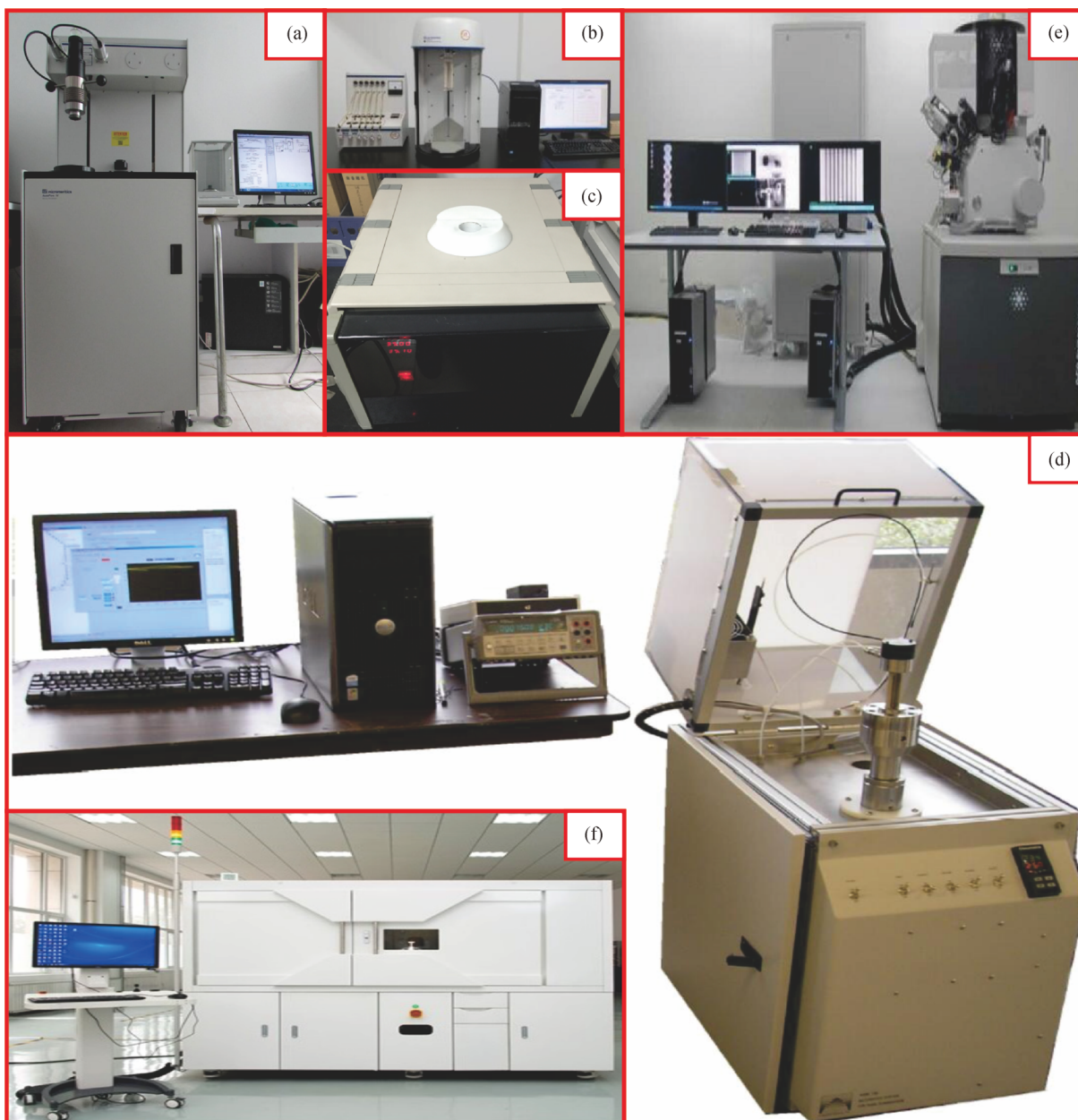
Fig. 3 Pictures of all the experimental facilities: (a) Autopore IV 9500 mercury injection apparatus; (b) automatic specific surface and pore analyzer Tristar II3020; (c) LF-NMR device RecCore-2500; (d) CMP device-APSE730; (e) double beam electron microscope system FEI Helio 650; and (f) NanoVoxel-3502 series X-ray three-dimensional microscope.
