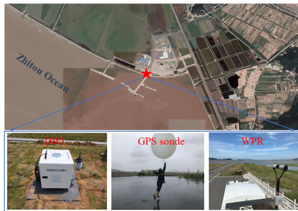
Fig. 2 Photographs showing the local surroundings of the field experiment site and relevant observational instrumentation comprising the DWL, GPS sonde, and WPR.
