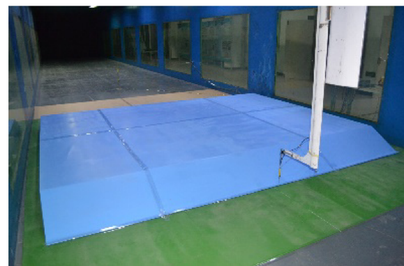
Fig. 1 (a) Sketches of the simplified 2D uphill terrain model with a limited length-upper surface of 7L . Aerodynamic characteristics at 5 locations along the slope surface and 11 points over each location along the slope surface were measured; and (b) the corresponding physical model in the wind tunnel with the Cobra Probes.
