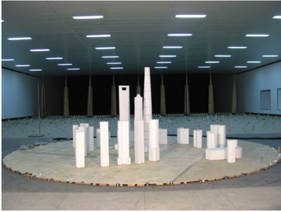
Fig. 2 Experimental investigation of the wind environment around tall buildings in AREA 1.
