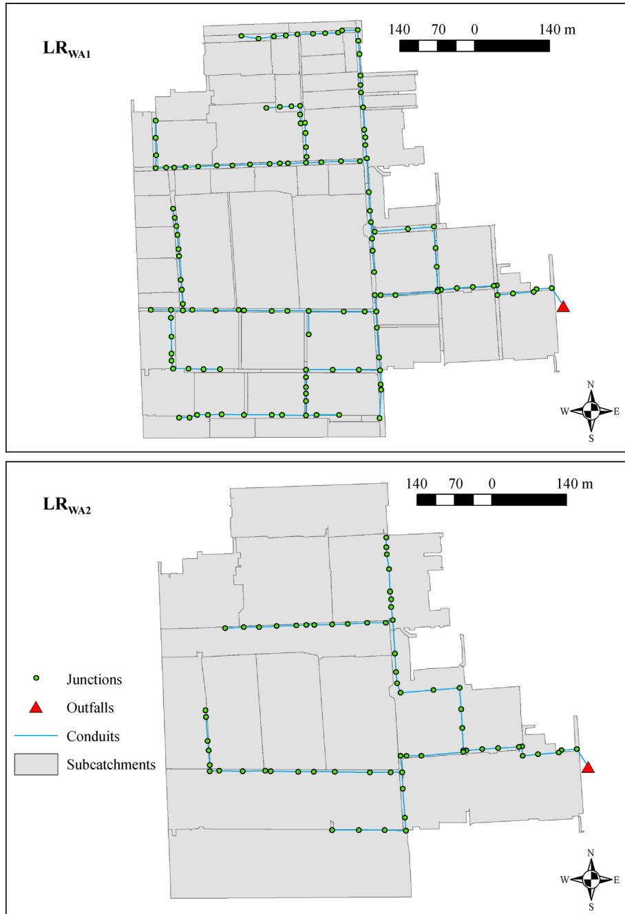
Fig. 3 The low resolution (LR WA1 and LR WA2 ) catchment discretization for the study area. Green dots indicate the sewer inlets, blue lines represent the storm water sewer network, and grey lines are subcatchment boundaries.
