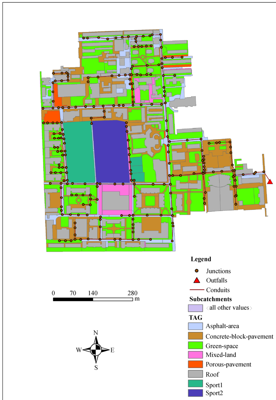
Fig. 2 The high resolution (HR) catchment discretization for the study area. Brown dots indicate the sewer inlets, wine red lines represent the storm water sewer network, and grey lines are subcatchment boundaries.
