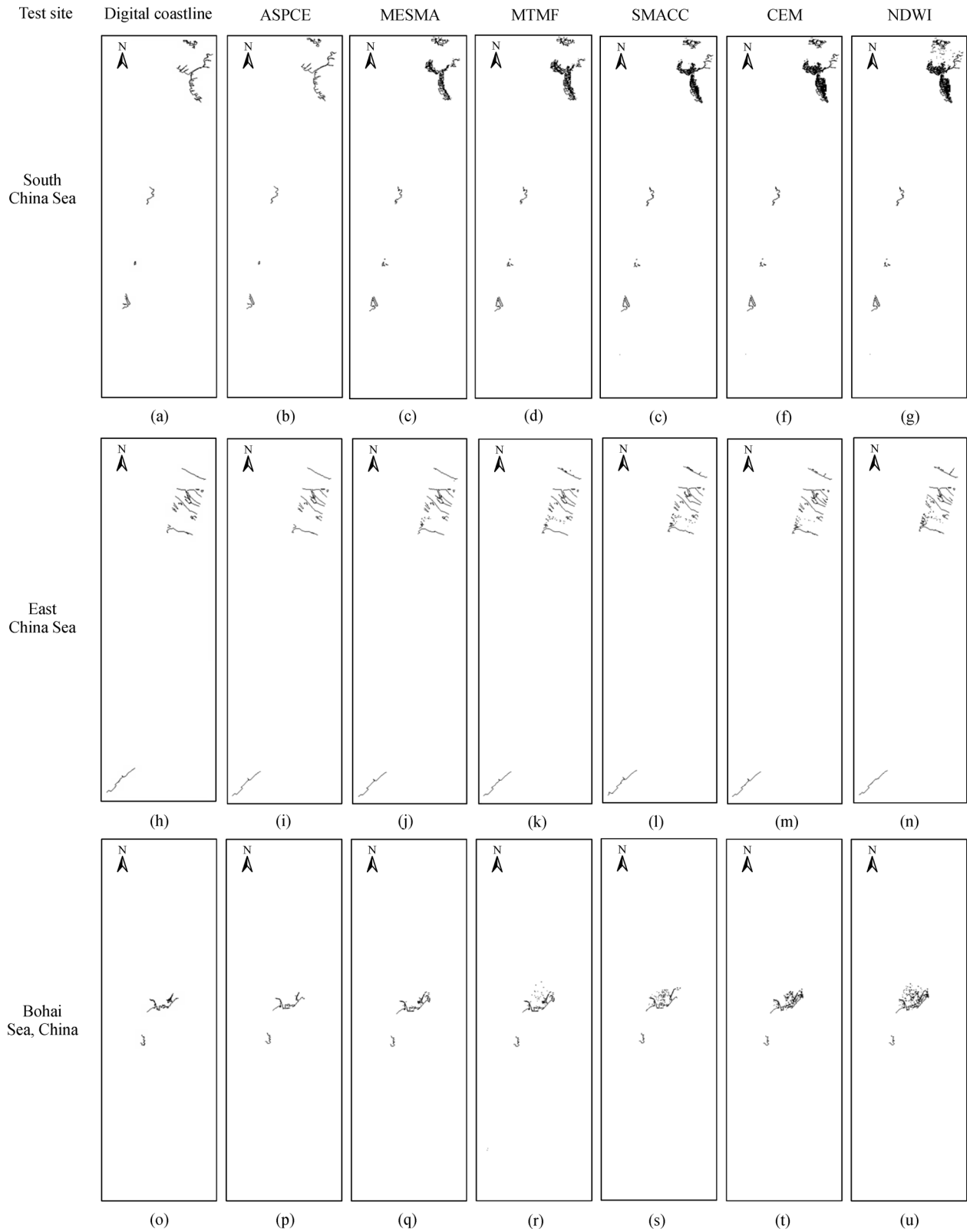
Fig. 8 Comparison of the coastline extraction results. First row, (a)–(g) are, respectively, the digital coastline and coastline extractions from the proposed method and the compared methods (MESMA, MTMF, SMACC, CEM, and NDWI) in the South China Sea; Second row, (h)–(n) are, respectively, the digital coastline and coastline extractions from the proposed method and the compared methods (MESMA, MTMF, SMACC, CEM, and NDWI) in the East China Sea; Third row, (o)–(u) are, respectively, the digital coastline and coastline extractions from the proposed method and the compared methods (MESMA, MTMF, SMACC, CEM, and NDWI) in the Bohai Sea, China.
