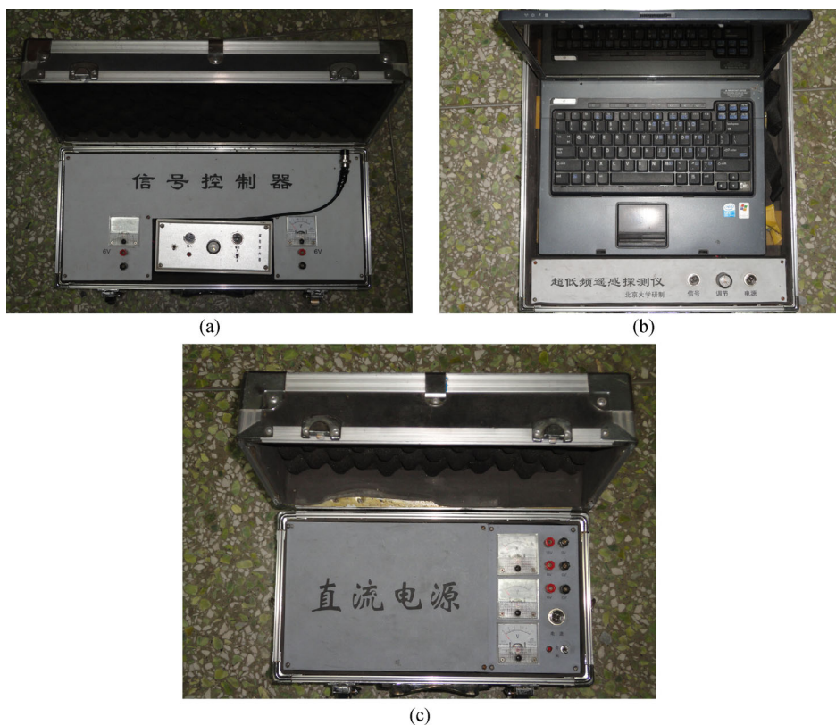
Fig. 7 Super-Low Frequency remote sensing system: (a) high-resolution remote sensor; (b) the processing unit; (c) the portable power supply.
