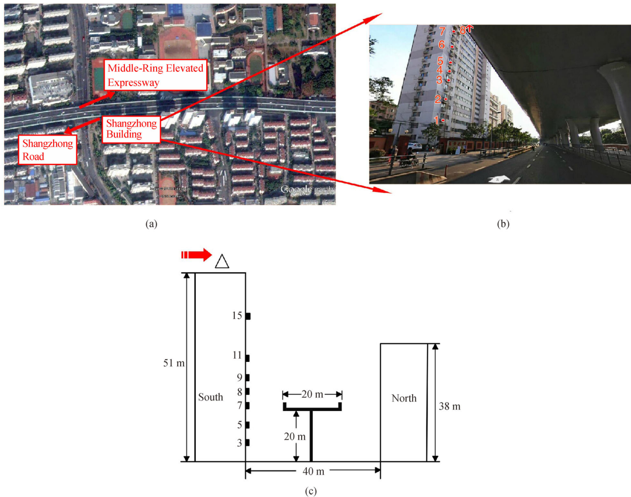
Fig. 1 Schematic of field measurement. (a) Field measurement site. (b) Shangzhong Building. (c) The distribution of monitoring sites in vertical section and within the street canyon.
