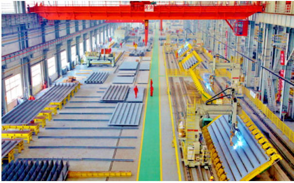
Fig. 5 Automatic production line of steel box beam plate unit of the bridge
