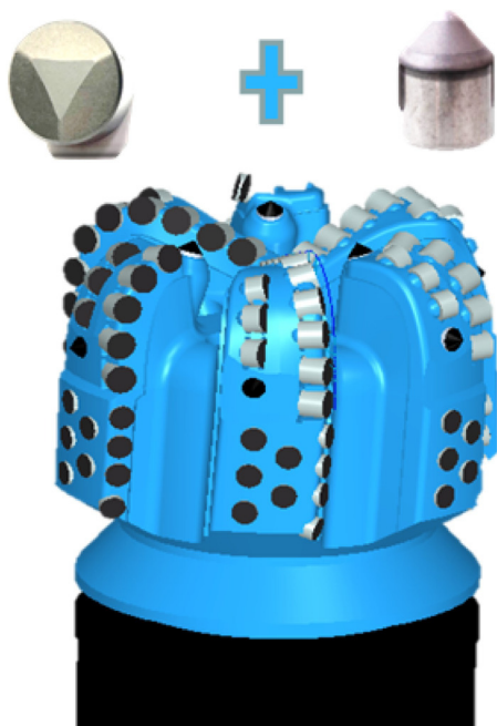
Fig. 5 Customized PDC bit design.
